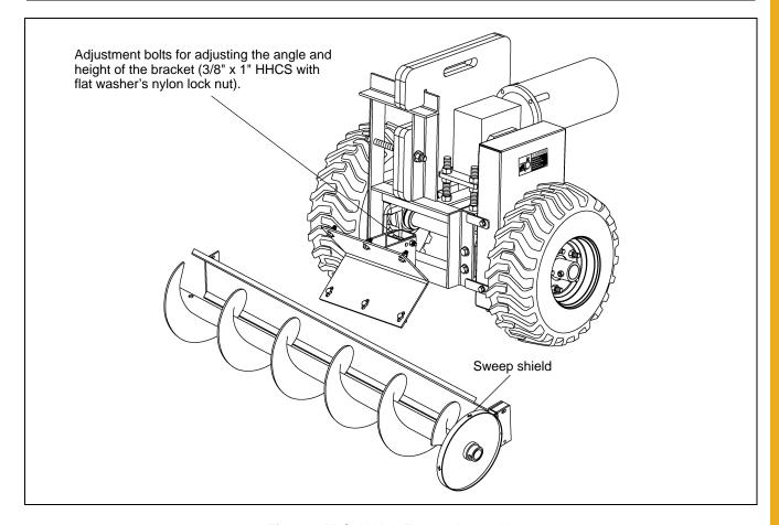
Figure 3M Shield to Tractor Assembly
